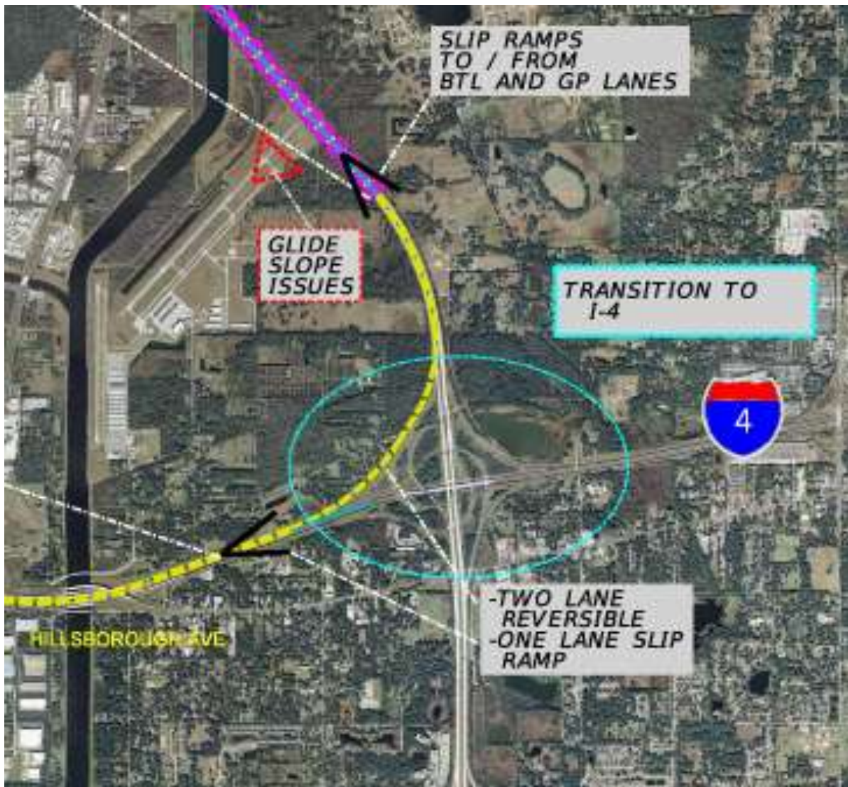
Figure D - 7: BTL#1 I-4 to I-75 North Connection (Reversible) Source: Parsons Brinckerhoff
