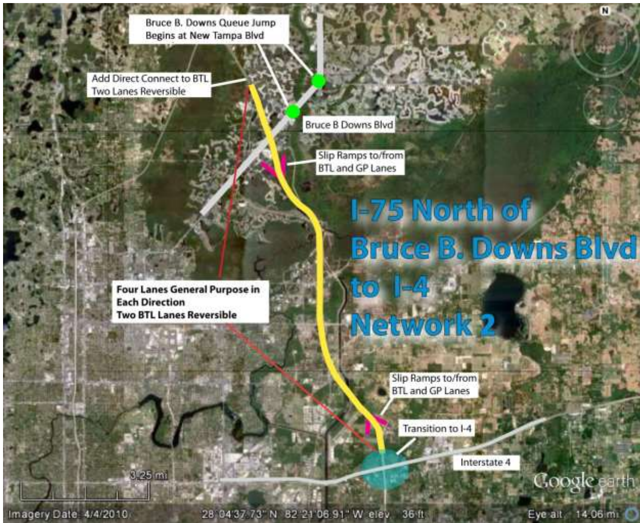
Figure C - 15: I-75 North with Direct connection to Bruce B. Downs Boulevard with Queue Jumps (Source: Parsons Brinckerhoff – Base Map Imagery © 2013 DigitalGlobe, The Florida Department of Environmental Protection, U.S. Geological Survey, Map Data © 2013 Google)
