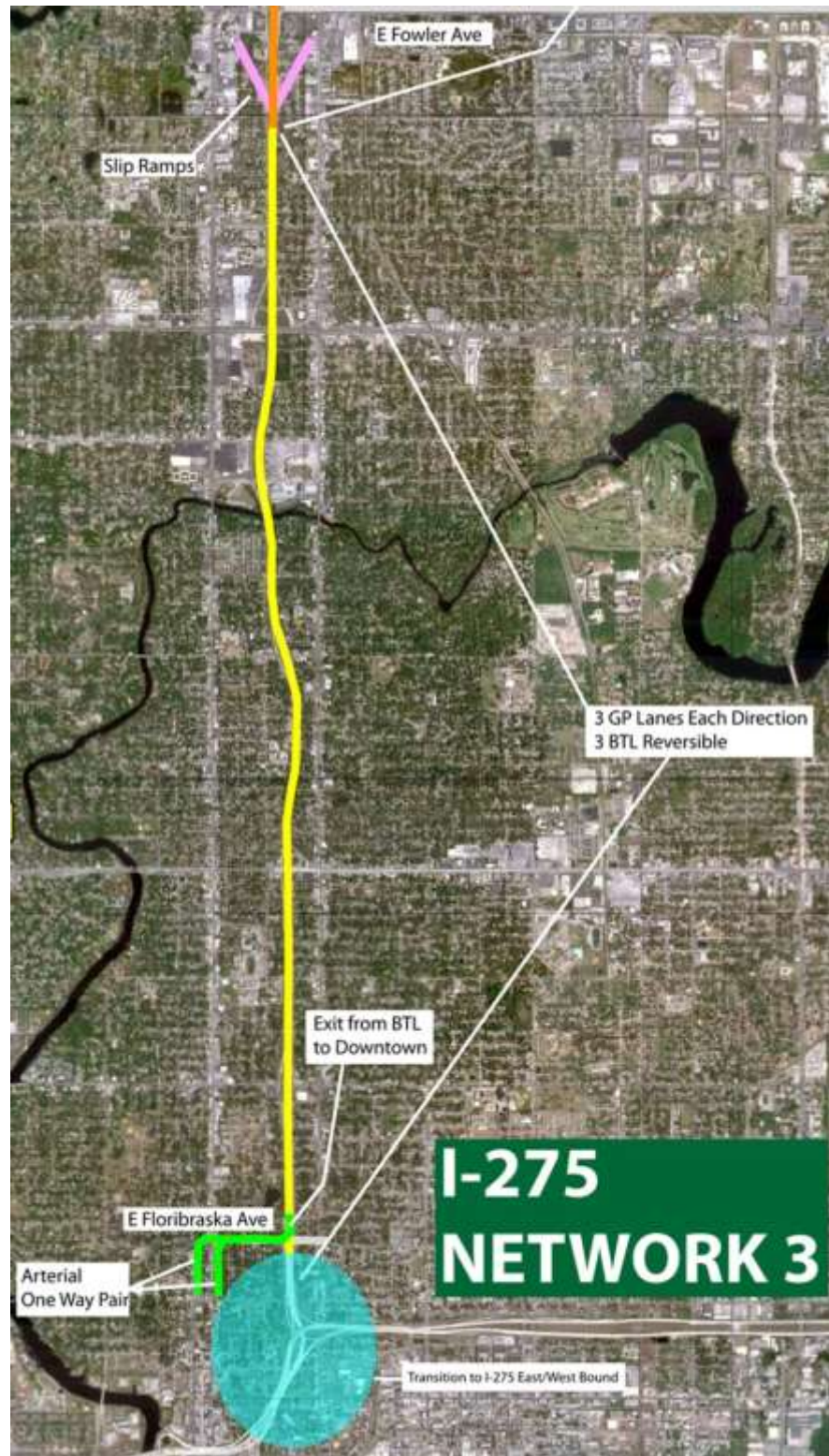
Figure C - 16: I-275 North Limited-Access BTL from Downtown Tampa to Fowler Avenue (Source: Parsons Brinckerhoff – Base Map Imagery © 2013 DigitalGlobe, The Florida Department of Environmental Protection, U.S. Geological Survey, Map Data © 2013 Google)
