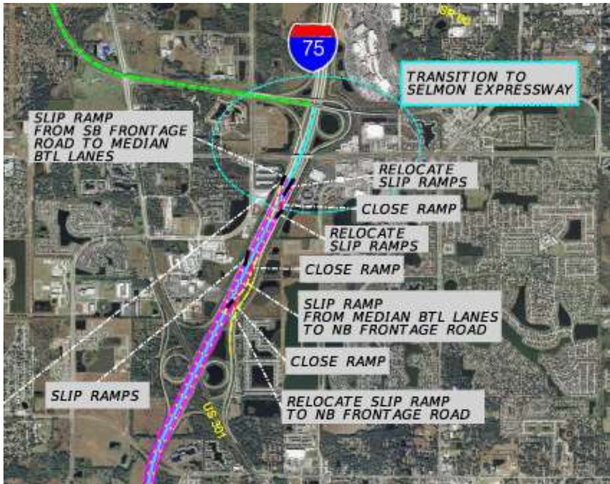
Figure D - 27: BTL#3 I-75 South Connection to Selmon Expressway (Reversible) Source: Parsons Brinckerhoff
