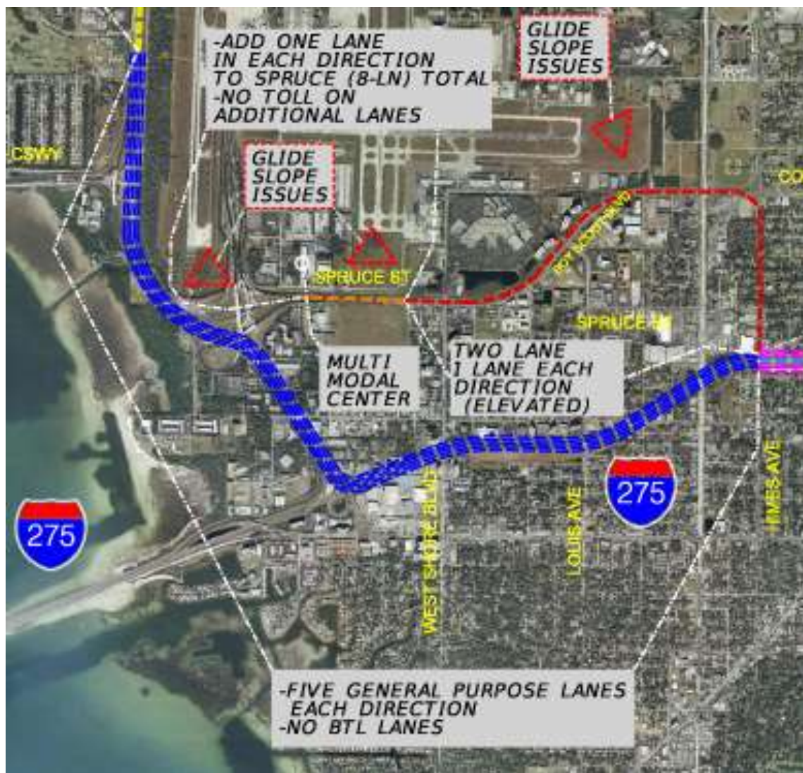
Figure D - 3: BTL#1 Airport to I-275 South BTL Connector (Combination of Arterial and Elevated 2-way) Source: Parsons Brinckerhoff
