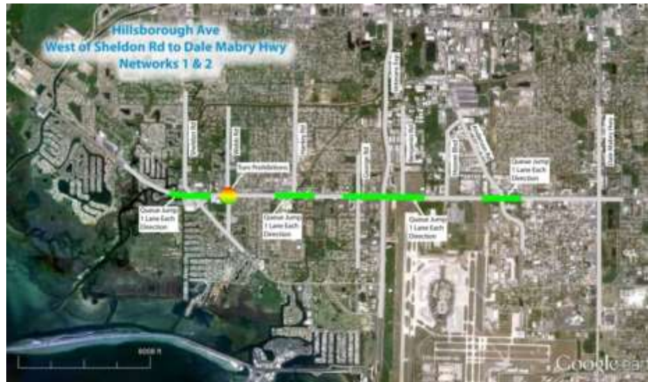
Figure C - 5: Hillsborough Avenue Arterial BTL Queue Jump Location (Source: Parsons Brinckerhoff – Base Map Imagery © 2013 DigitalGlobe, The Florida Department of Environmental Protection, U.S. Geological Survey, Map Data © 2013 Google)
