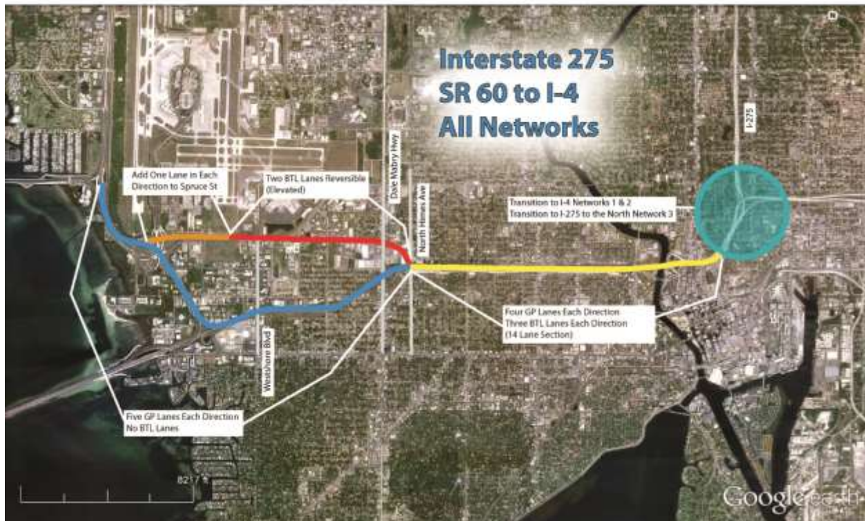
Figure C - 4: I-275 Limited-Access BTL Between Tampa Airport and Downtown Tampa (Source: Parsons Brinckerhoff – Base Map Imagery © 2013 DigitalGlobe, The Florida Department of Environmental Protection, U.S. Geological Survey, Map Data © 2013 Google)
