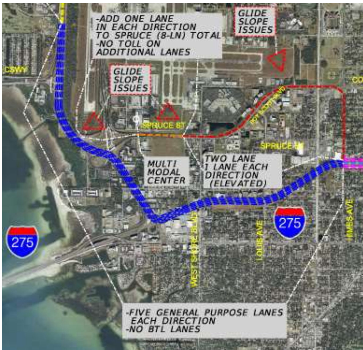
Figure D - 21: BTL#3 Airport to I-275 South BTL Connector (Combination of Arterial and Elevated 2-way) Source: Parsons Brinckerhoff
