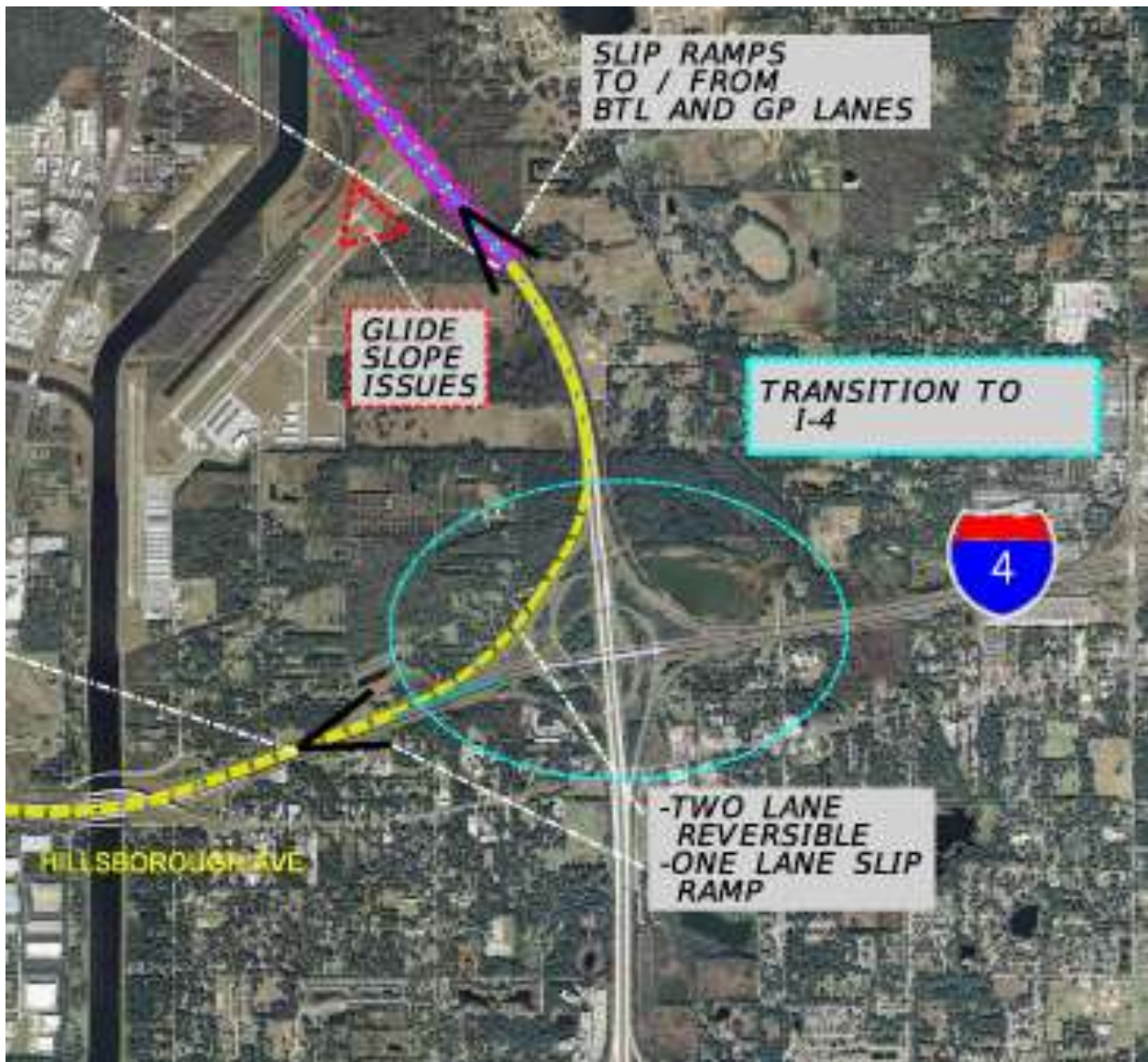
Figure D - 18: BTL#2 I-4 to I-75 North Connection (Reversible) Source: Parsons Brinckerhoff
