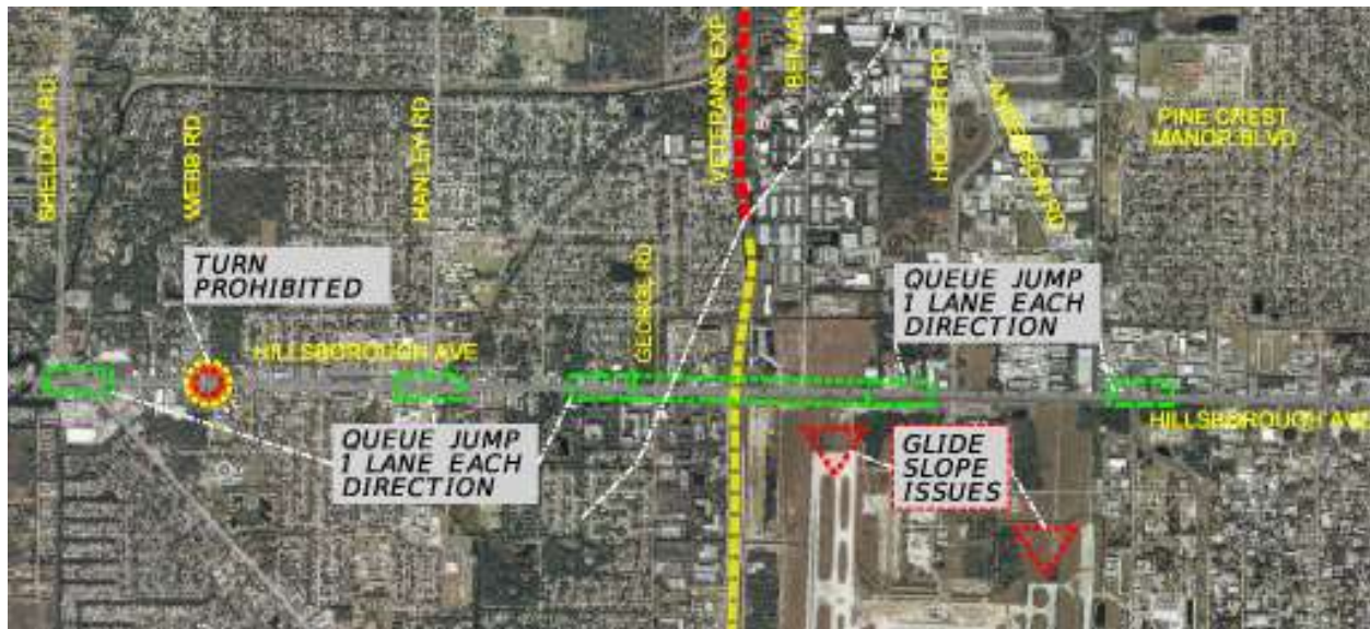
Figure D - 14: BTL#2 Hillsborough Avenue Arterial Queue Jumps (2-way) Source: Parsons Brinckerhoff
