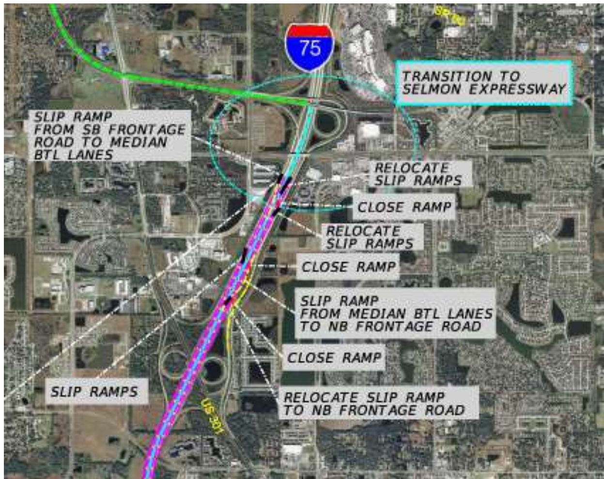
Figure D - 11: BTL#1 I-75 South BTL Connection to Selmon Expressway (Reversible) Source: Parsons Brinckerhoff
