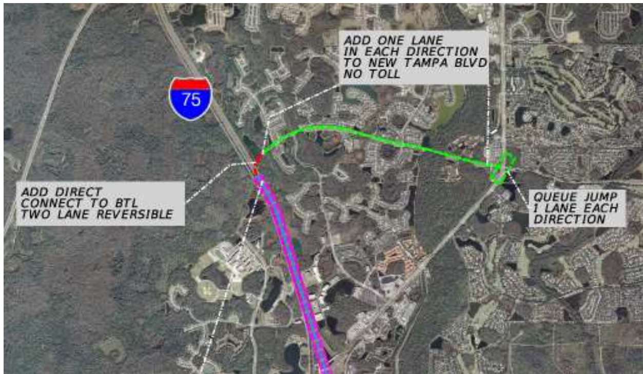
Figure D - 9: BTL#1 I-75 North BTL Connection to New Tampa Boulevard (Source: Parsons Brinckerhoff)
