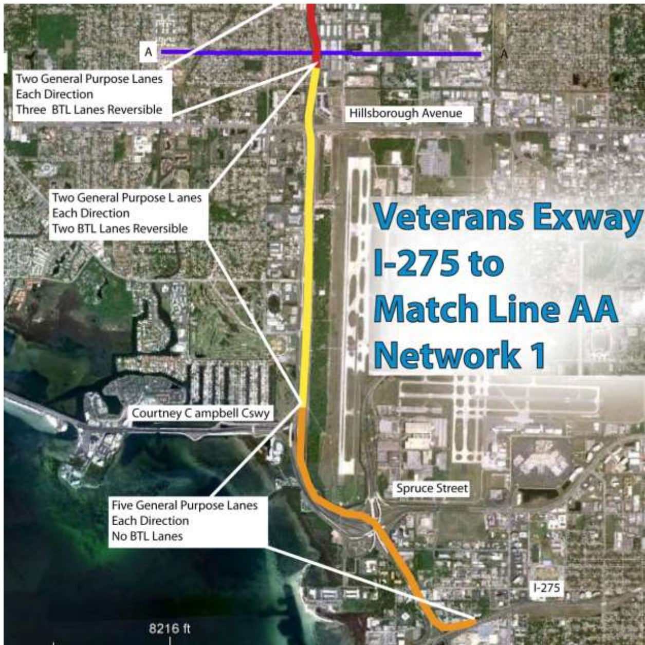
Figure C - 9: Veterans Expressway Limited-Access BTL from I-275 to North of Hillsborough Avenue (Source: Parsons Brinckerhoff – Base Map Imagery © 2013 DigitalGlobe, The Florida Department of Environmental Protection, U.S. Geological Survey, Map Data © 2013 Google)
