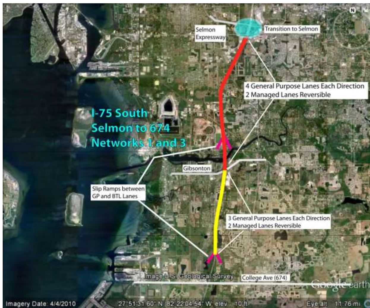
Figure C - 7: I-75 South Limited-Access BTL from SR 674 to the Selmon Expressway (Source: Parsons Brinckerhoff – Base Map Imagery © 2013 DigitalGlobe, The Florida Department of Environmental Protection, U.S. Geological Survey, Map Data © 2013 Google)
