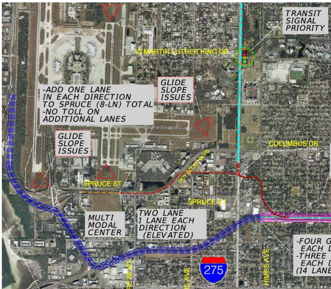
Figure D - 13: BTL#2 Airport to Dale Mabry Highway to I-275 South BTL Connector (Combination of Arterial and Elevated 2-way) Source: Parsons Brinckerhoff
