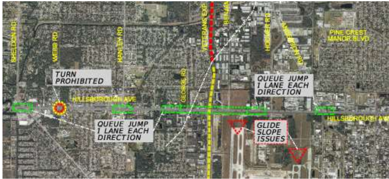
Figure D - 2: BTL#1 Hillsborough Avenue Arterial Queue Jumps (2-way) Source: Parsons Brinckerhoff
