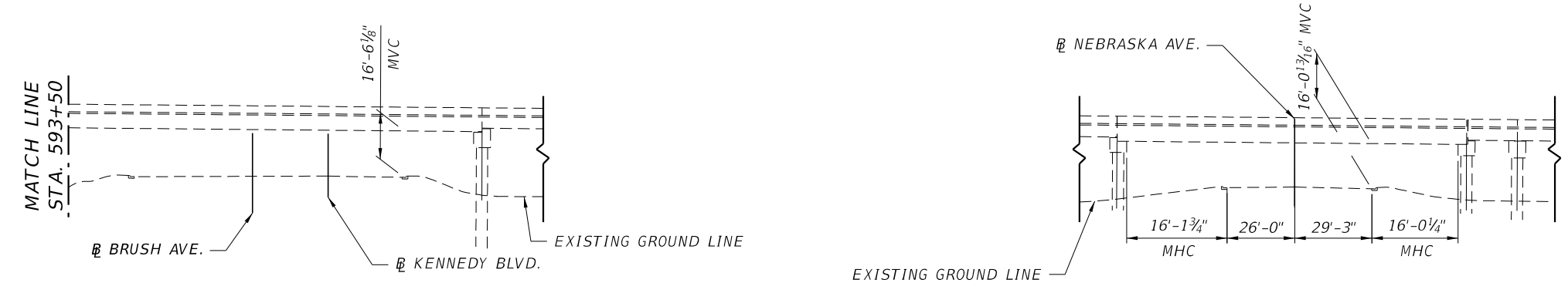
EASTBOUND ELEVATION SELMON EXPRESSWAY DOWNTOWN TAMPA VIADUCT OVER KENNEDY BOULEVARD, BRUSH AVENUE, AND NEBRASKA AVENUE NTS
